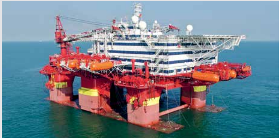
Keppel FELS delivered Floatel Triumph, the fifth high-specification accommodation semisubmersible built to Keppel's proprietary SSAU™5000NG design, safely and on time
