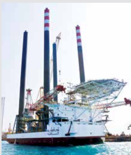
Al Safliya, the first liftboat to be wholly constructed in Qatar, is built to the ORCA 2500 design developed by Keppel O&M's design arm, Bennett Offshore
